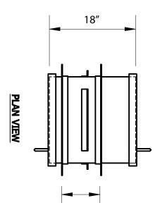
FRAME ADJUSTABLE FOR 3-1/2"-8" WALL THICKNESS
