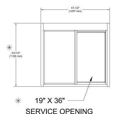
275 - 43-1/2" H GLAZING ROUGH OPENING = 47-3/4" W (1213 mm) x 43-3/4" H (1111 mm) MASONRY ROUGH OPENING = 48" W (1219 mm) x 44" H (1118 mm)
