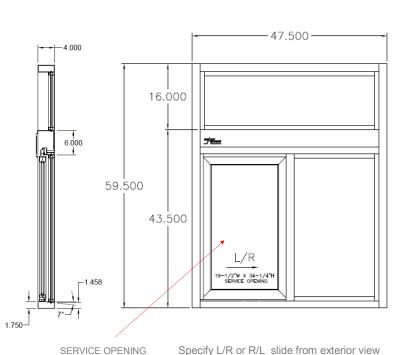
All windows are shipped completely pre-assembled, fully glazed and ready to install.
