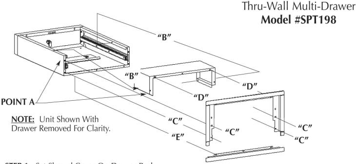
STEP 1: Set Shroud Cover On Drawer Body Holding The Front Of Shroud & Front Of Drawer Housing Flush (REF POINT A). Mark The Slot Location On The Inside Of The Housing & Drill .136 DIA. (#29 Drill) Hole In Housing (REF "B").
